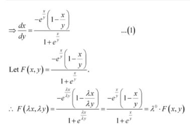
Therefore, the given differential equation is a homogeneous equation.
